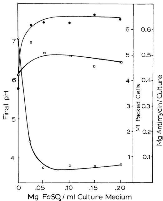
FIG. 1. Effect of iron on antimycin production. Initial pH = 7.2; 100-ml cultures in 250-ml shake flasks. Symbols: ●, terminal pH; □, packed-cell volume; ○, antimycin (in mg/culture).
