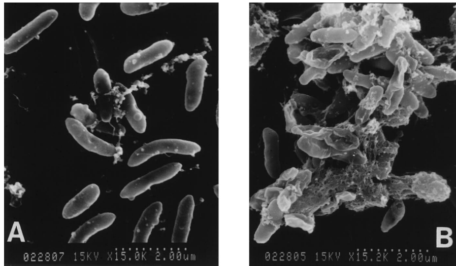
FIG. 1. Scanning electron micrographs of P. aeruginosa 2126 on the surface of Teflon sheets incubated for 1 day (A) or 6 days (B).
