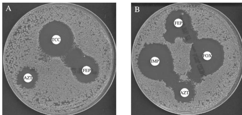
FIG. 1. Double-disk synergy test with *bla*<sub>VEB-1</sub>-positive *P. stuartii* strain BI on MH agar plates with clavulanate (A) or imipenem and ceftoxitin (B) as inhibitors. The disks tested contained ticarcillin plus clavulanate (TCC), imipenem (IMP), ceftoxitin (FOX), cefepime (FEP), and aztreonam (AZT).
