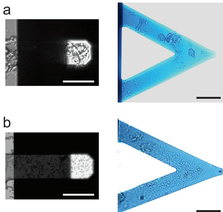
**FIG 8** Optical images of bacterium-bearing sensors. Typical optical images of rectangular (left panels) and triangular sensors (right panels) bearing BCG (a) and *M. abscessus* (b). The optical images show the BCG clumping. Scale bars, 50  $\mu\text{m}$ .
